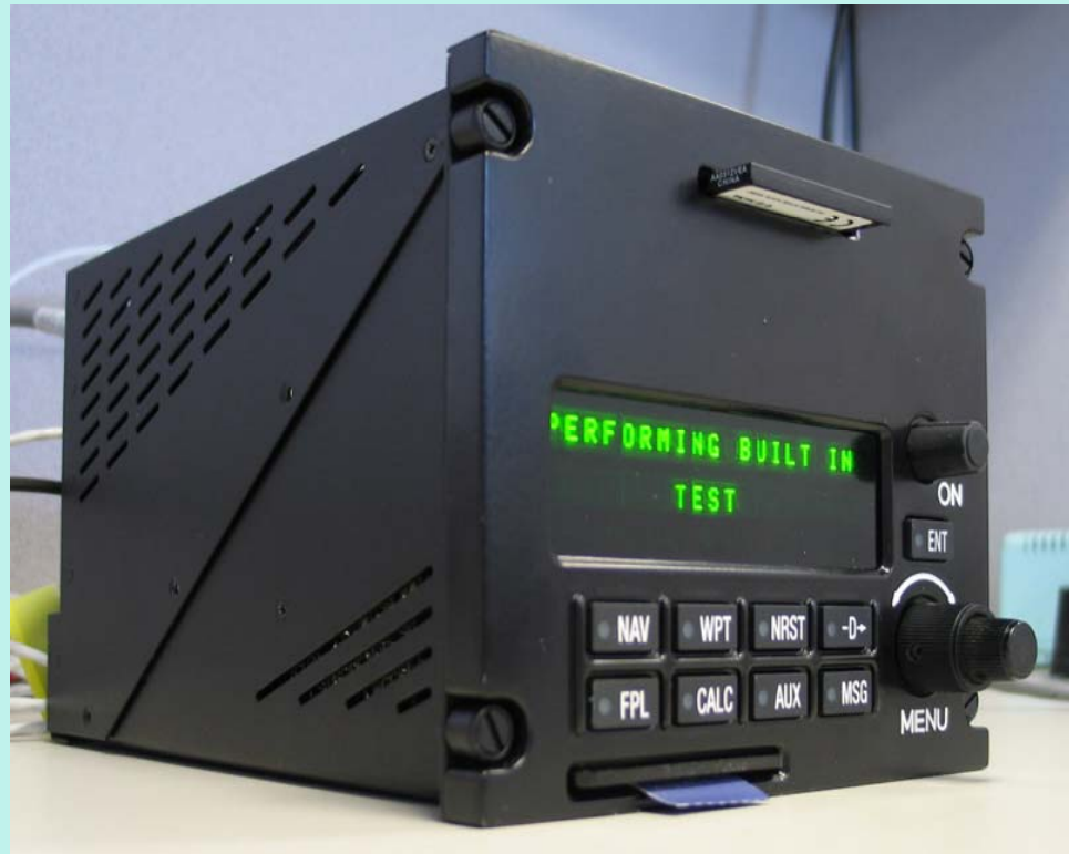
Figure : Combined GPS/Loran Navigation unit
